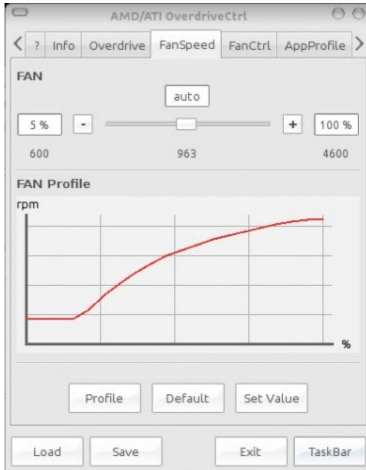
On this tab you can set a fixed fan speed. The possible range is again delivered by the ADL.
